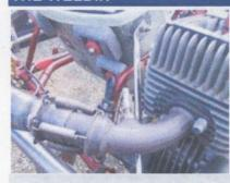
To be fitted preferably, on the inside of a bend, or, in the primary divergence cone of the exhaust system (primarily for very high performance engines i.e., CIK reed and rotary engines). It must be sited far enough from the engine, so as not to get too hot, but as it needs to reach 300 to 350 degrees C or higher, (not too much higher), it can't be too far away.
