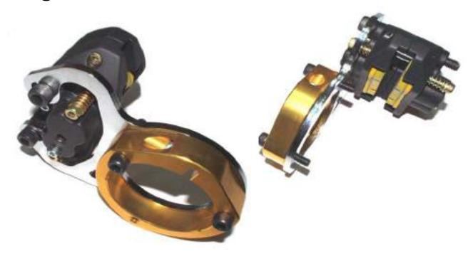
The caliper mounting bracket is designed to bolt to the rear axle bearing mounting bolts, 30 mm, 40 mm & 50 mm bearing configurations.
