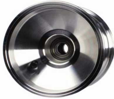
5" DIA X 100mm WIDE EXTRA O/SET SOLD AS WET TYRE WHEELS
