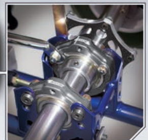
40mm axle supported by three bearings
