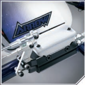
Machined billet alloy brake master cylinder anodised black
